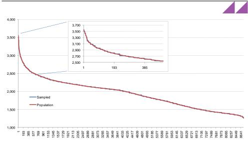
Figure A1 Comparison of 100 point sampled LDC with hourly trace (MW)
