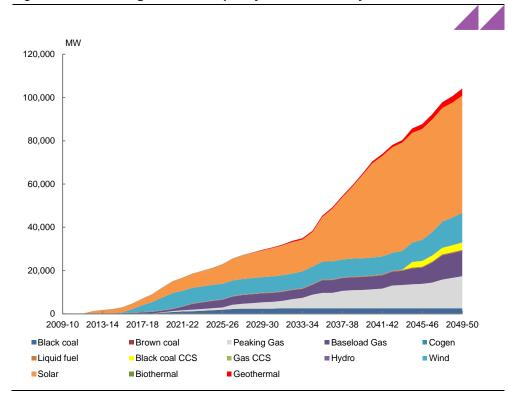
Figure 26 Installed generation capacity - Central Policy scenario
