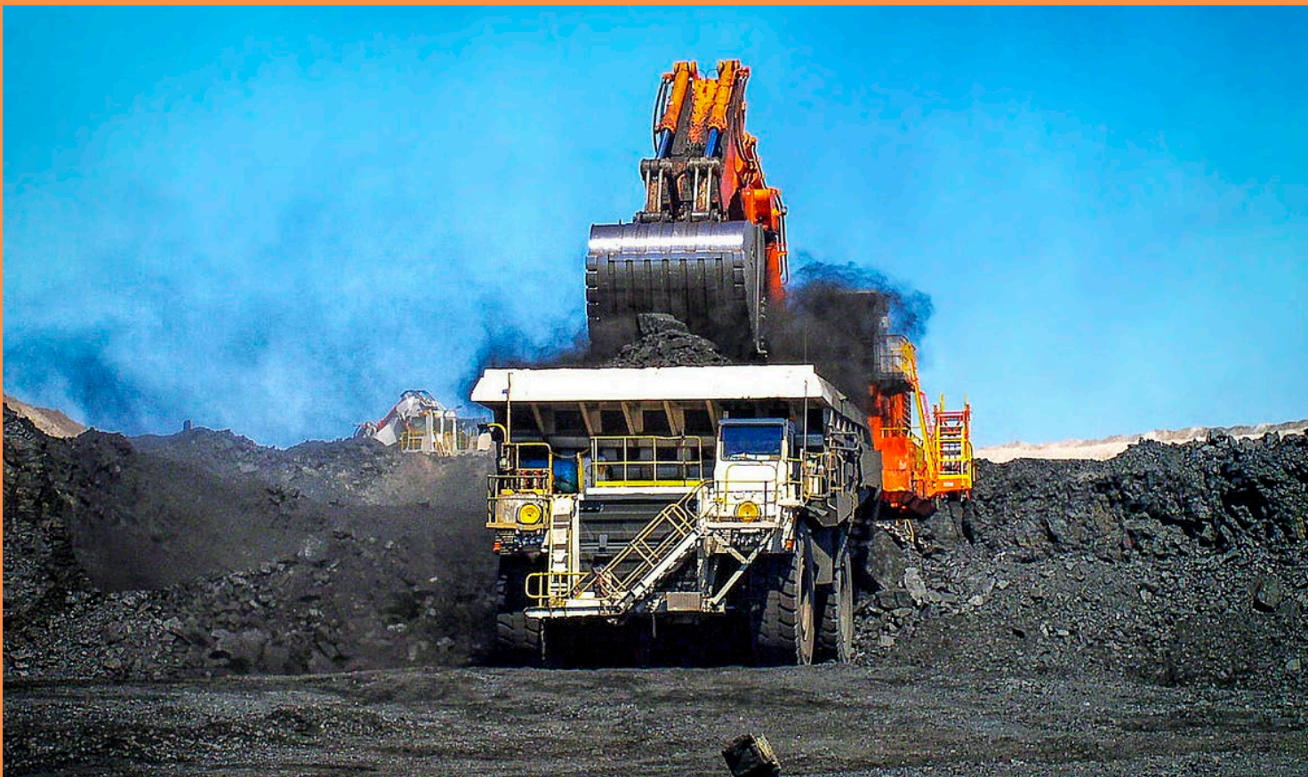
A large excavator loads black coal into a heavy dump truck at an open cut mine in Queensland.
